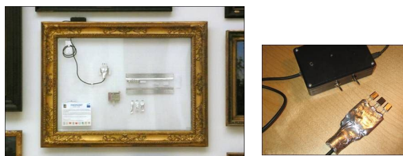
Figure 5 Sample holder adapted for monitoring within paint frames is shown on the left (control box is placed outside the frame and is on top of the frame). Detail of the holder and control box, which also contains the batteries, is shown on the right. Paint frame was located in the Statens Museum (Copenhagen) and exposure made during the PROPAIN project
