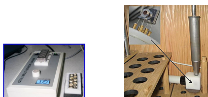
Figure 2 Powered unit (QTS-3) used in the MIMIC project for continuous monitoring (left) and adapted crystal holder for monitoring environment within organ pipes (right) as mounted in St Botolph without Aldgate (London).
