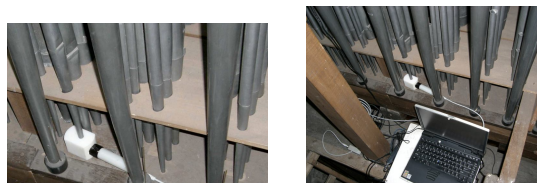
Figure 4 The sample holder as set up in the organ in the cathedral in Olkusz (Poland) (left) and the full setup including the PC (right)
